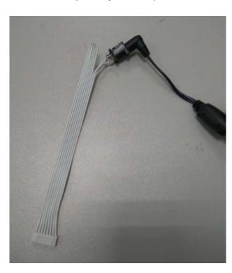
Note: If you need to use this method, we can help to provide this type cable soldered with a power jack, see below picture.
