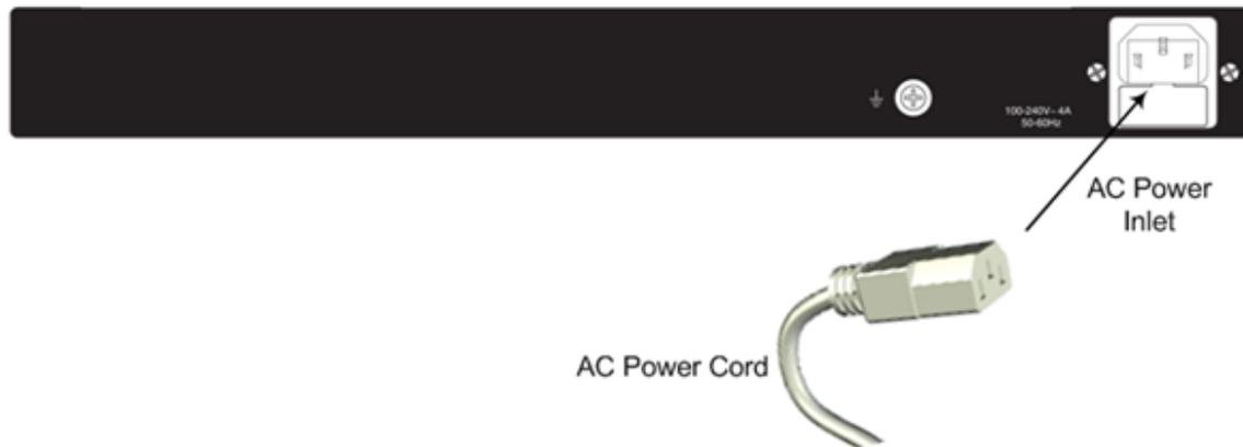
2. Connect the plug at the other end of the AC power cord to a standard electrical outlet.
