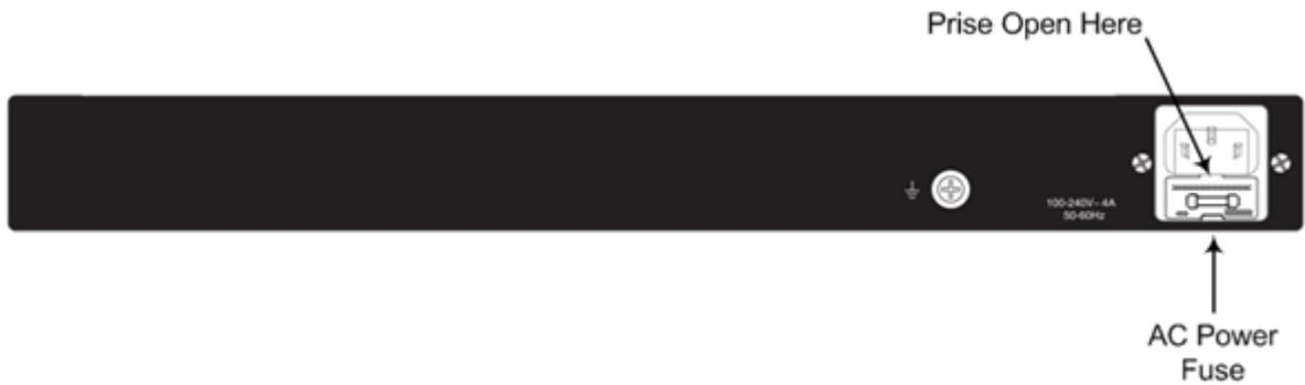
3. Carefully remove the fuse from the fuse cavity.
