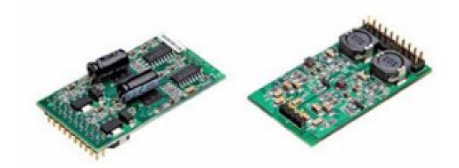
The FXS (Foreign Exchange Station) port is an interface that connect to a station, such as an analog telephone or the FXO interface of another
