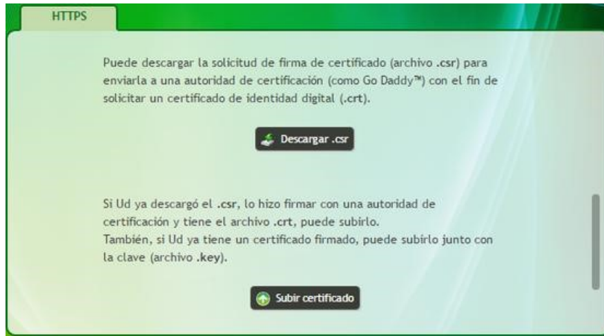
Figure 3.113: Web server, certificate download and import
