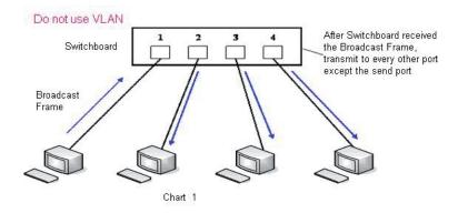
Chart 1 shows a network switch with no VLAN. Any broadcast frames will be transmitted to all other ports. For example, and frames broadcast from Port 1 will be sent to Ports 2, 3, and 4.
